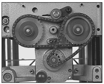
Figure 33. Location of sprocket bolts.
